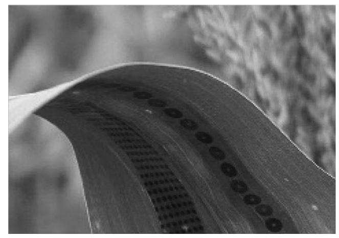
Engineers have made wearable sensors for plants, enabling measurements of water use in crops.
